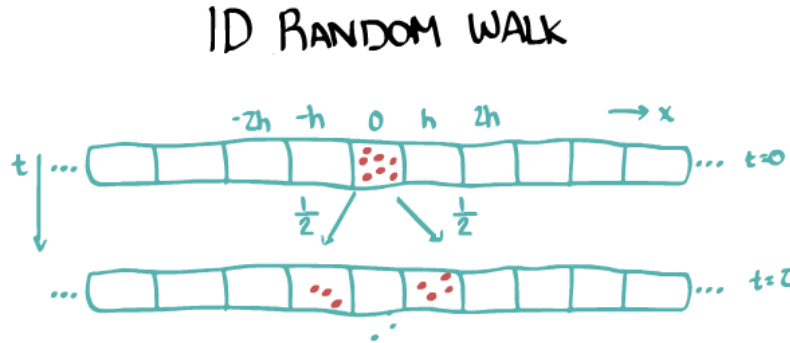
FIGURE 2. Random Walk. This figure illustrates a cartoon schematic of random walks along a one-dimensional lattice in the case where particles move right and left with equal probability.
